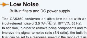
improve the signal-to-noise ratio (SN ratio), the built-in filter can be set to a response speed in the range of 1 µs to 300 ms to optimize the SN ratio and response speed depending on the application.
